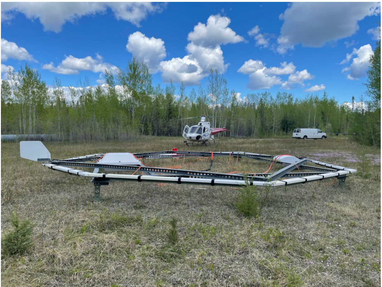
Figure 4: Airborne system used for the Boulder Airborne Survey.
