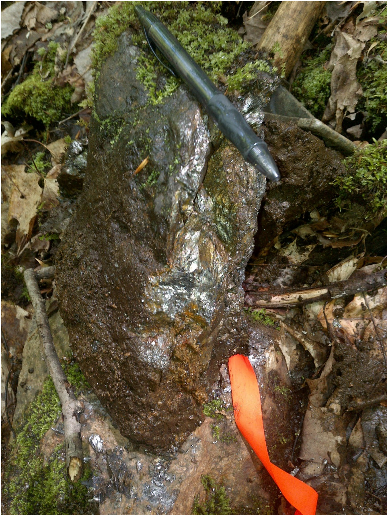
Figure 8: New graphite mineralization found with Beep Mat.
